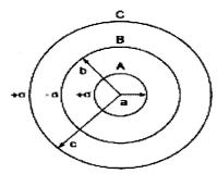
If shells A and C are at the same potential, then obtain the relation between the radii a, b and c.
